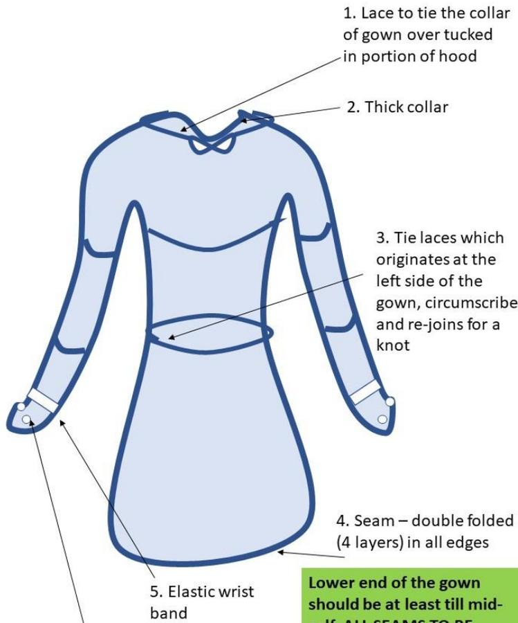
**Lower end of the gown should be at least till mid-calf, ALL SEAMS TO BE DOUBLE FOLDED AND STITCHED properly for prevention of any leakage**
