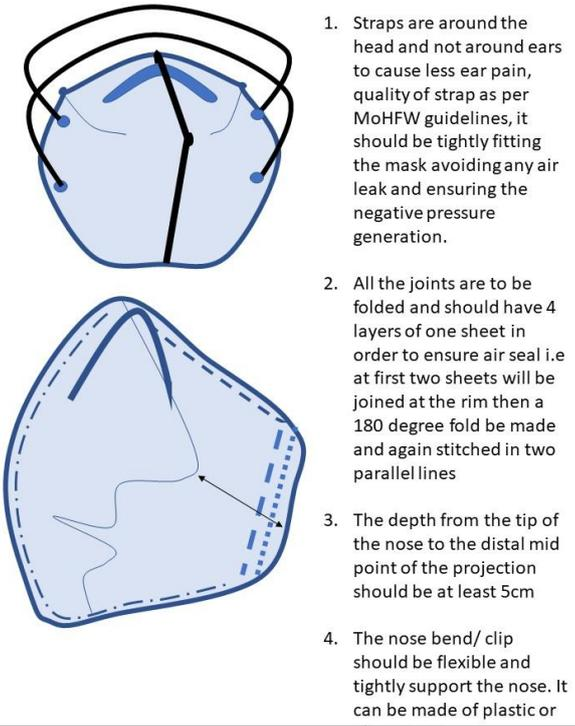
**Fig 3: PPE face mask (O2 ply), seams are double folded and properly stitched with nose clip**
