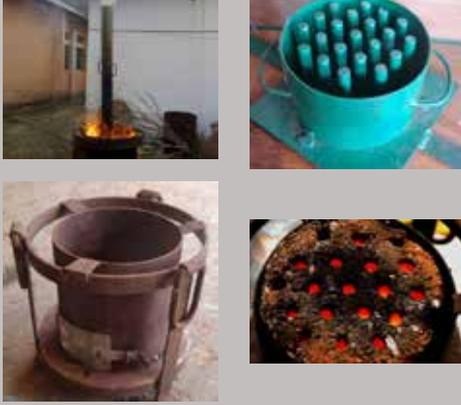
The Innovation is production of beehive charcoal briquettes from waste biomass for cooking and space heating in rural areas. The development included a charring kiln, a beehive briquetting mould and a beehive briquette stove.
